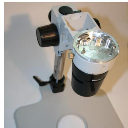
Fig. 3. Placement of the Condenser Support Bracket on the Post
