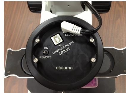
Fig. 7. Power/Signal Phase Cable for Phase Contrast Accessory operation with LS 620/600.
