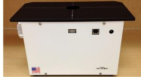
Fig. 6. Back of Lumascope 500/400, showing USB port into which the LS 500/400 Phase Signal Cable is inserted.
