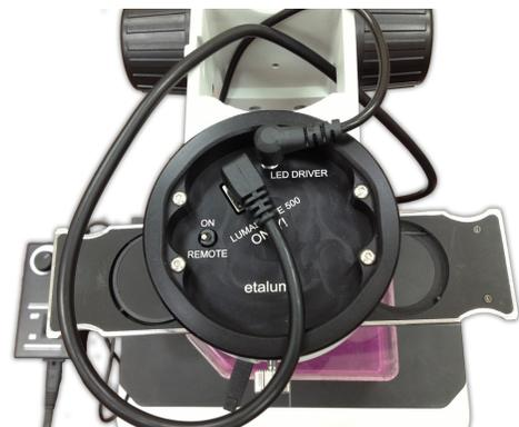
Fig. 5. Cables and controls for Phase Contrast Accessory operation with LS 500/400.
