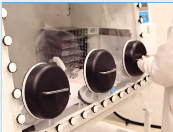
Removable front cover with triple glove ports makes the SCI-tive easy to use.
