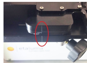
Fig 7. Alignment marks on LS720 plate carrier and top deck on instruments with subdeck Version 2
